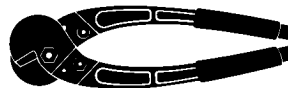
Wire cutters - only needed if you are cutting your own headstay wire
