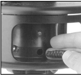
When replacing line, pass it through enclosed opening in guard. Pass line into hole in hub of spool. Pull line down from below and clamp on a HCP237 "hog ring". Pull back to tighten.
