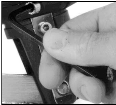
Use the provided 5 mm allen wrench to loosen the two line guard screws.
