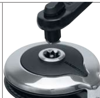
A Harken® locking handle inserted into an unloaded winch automatically disconnects the motor gear for manual operation
